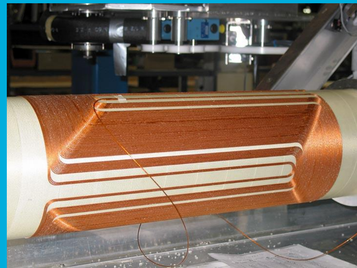
(Fig. 1: A direct-wind magnet being wound at BNL (1))
